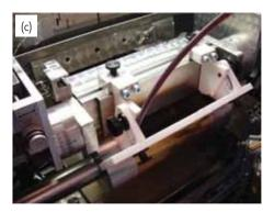
Fig. 6 (a) Photograph of the standing meniscus during slot-die coating of the active layer of the OPV comprising many very tightly spaced stripes. (b) A total of 48 stripes (3 mm wide spaced by 1 mm) are coated simultaneously). (c) Knife coating with the open ink reservoir and the manual feed hose.
