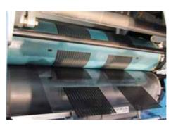
Fig. 4 Flat-bed screen printing of silver paste showing the squeegee after passage over the motif (left) and the squeegee during a printing cycle showing how the ink is forced through. The printed motif can be seen in the lower part of image (middle). A photograph of rotary screen printing of conducting graphite ink onto a clear polyester foil (right).
